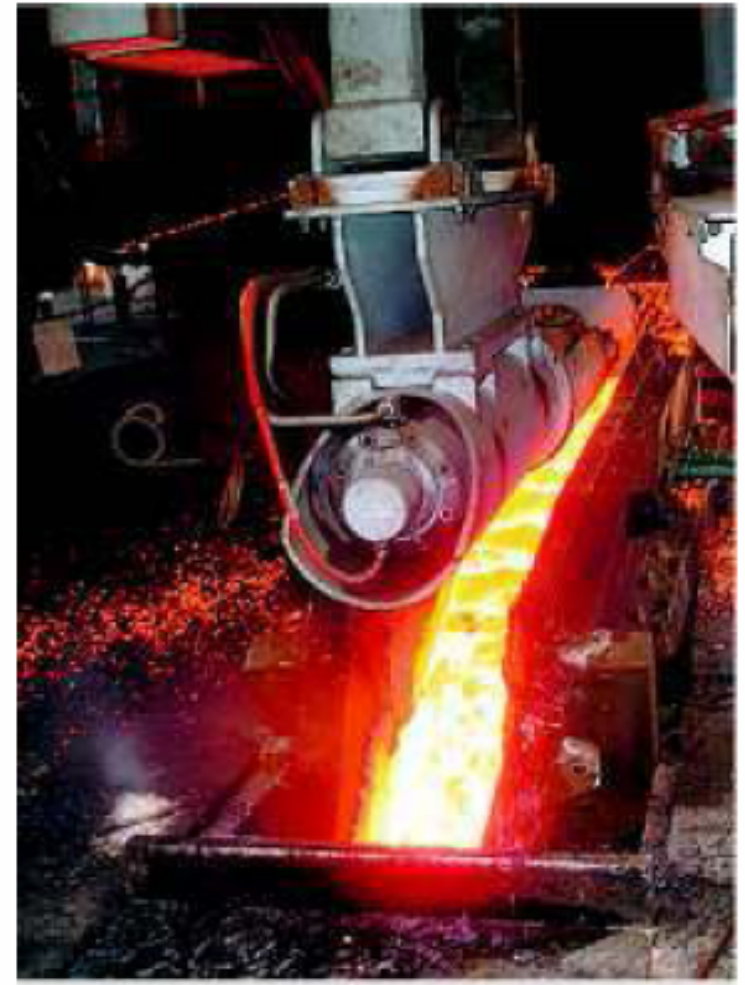
SAFE ... ISASMELT in operation
